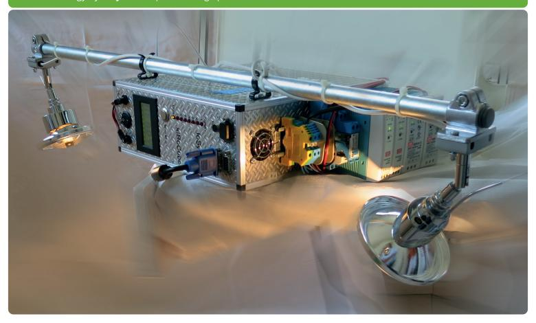
With the near infrared spectrometry (NIR) of the IoSys units it is possible to identify bigger plastic parts of the household-, engineering electronics fields. It allows direct analysis of non-dark-colored plastic parts and other materials like carpets and textiles.
