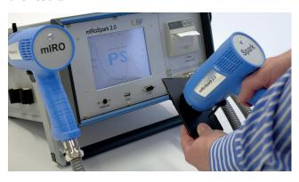
The identification of different plastic types for both spectrometers is the result of a trained pattern recognition with a specially developed neural network inside a database with several counterchecking. The result of the calculation is a list of the most probable polymer types identified within a probability between 0 and 100%. This comparison is necessary, since – contrary to metals – plastics have no norms and no standardizations!
