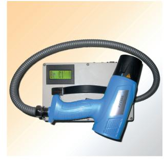
The portable sliding spark spectrometer allows the following samples to be analyzed within 1 second and independently of colour:
